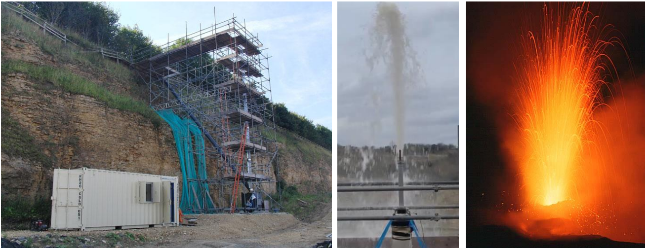
Figure 1. Left) The Large Analogue Volcano Apparatus (LAVA); middle) analogue eruption of LAVA; right) eruption of Stromboli, Italy (from Stromboli online).
